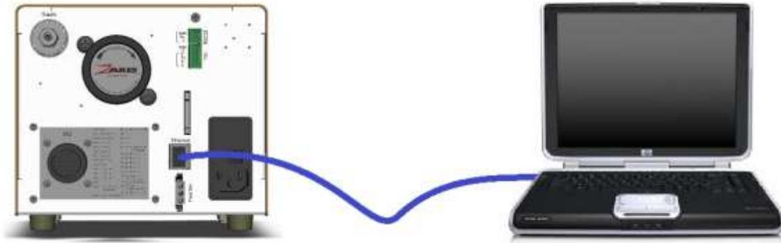
The setup data from on the Isaac can be modified by a computer via the Ethernet connection on the back of the Isaac.
