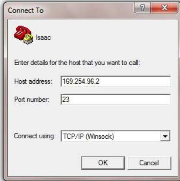
Pressing OK will initiate the socket connection from HyperTerminal to the Isaac. A successful connection will be show by the connected counter in the lower right corner of the HyperTerminal screen.
