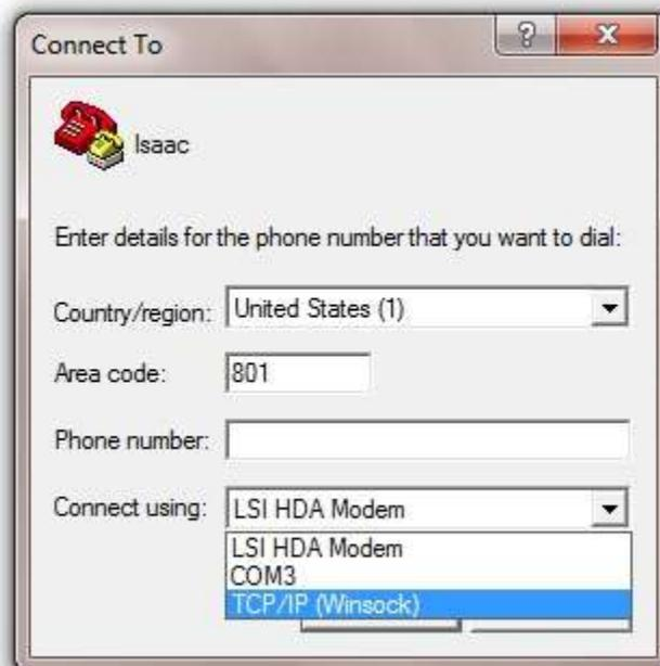
With the TCP/IP selection made the Host address and port numbering must be entered. The IP of the Isaac is the Host. The port number is always 23.
