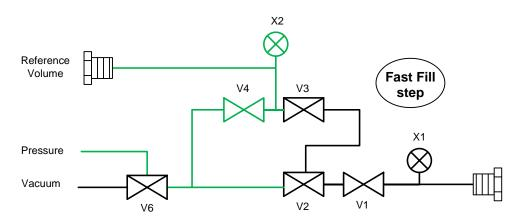
During the **fill** timer, the volume of pressurized air is sent to the test port. This pressure is monitored by (X1). The change in total volume will cause a pressure drop from the initial charge. With a good part in the test chamber, the target pressure will be achieved.
