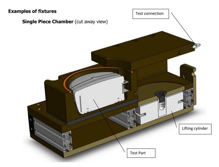
The part is loaded into the nest and slid into the test position. The lifting cylinder seals the test chamber against the top plate.
